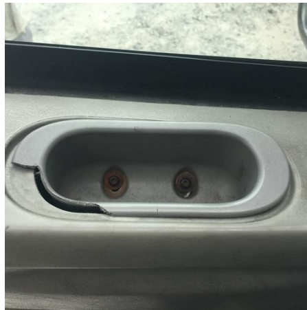
Door handle is broken
