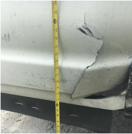
Crack in the passenger side
